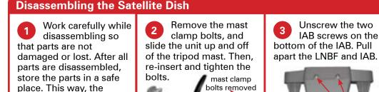
satellite dish can easily be reassembled at another time or location. bottom of IAB Loosen the two IAB Pull apart the IAB so 6 7 hex nuts on the top that the two parts are no longer attached to of the IAB. Remove the the LNBF arm. two IAB bolts and the two IAB hex nuts.
